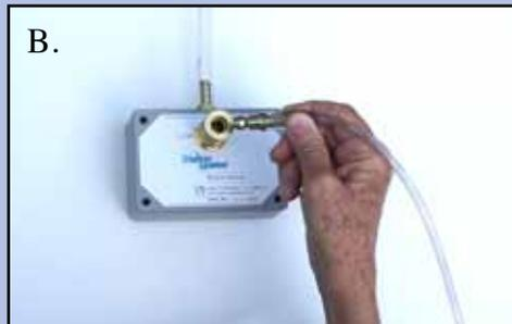
needed to engage or disengage the cannula coupling from any of the system's "Oxygen Out" connectors.
